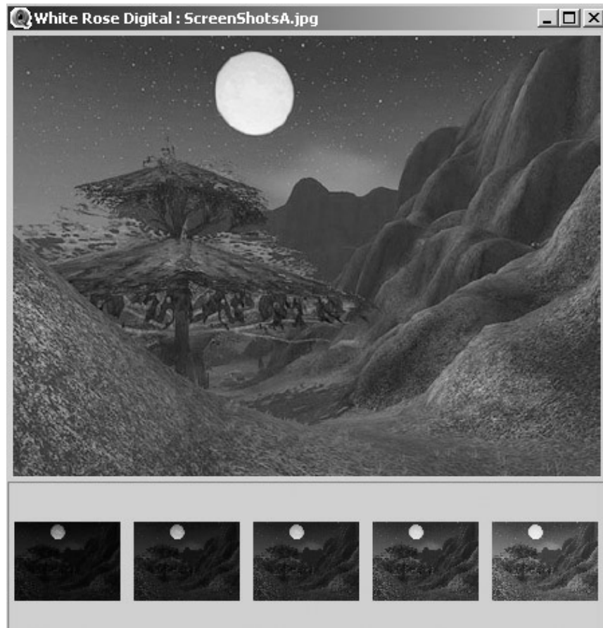
Figure 2. An illustration of the five-images-at-a-time user-choice methodology, as applied to a hierarchy of brightness and contrast intervals [1, 2], where each of the brightness and contrast choices are typically part of a three-stage hierarchy varying from coarse, through medium to fine (a single JAVD).
