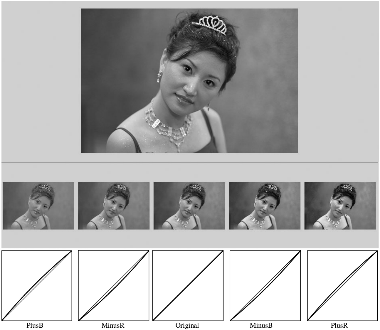
Figure 4. The user-choice images provided for image color correction, allowing an appropriate color change to be compared to the original (center).
